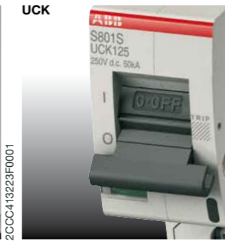
Tripping characteristics UCK Thermal tripping 1.05...1.2 \cdot I_n Electromagnetic tripping 11 \cdot I_n DC Calibration temperature 40^\circ\text{C}
