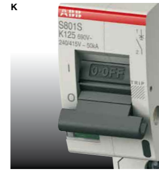
Tripping characteristics K Thermal tripping 1.05...1.2 \cdot I_n Electromagnetic tripping 13 \cdot I_n AC Calibration temperature 40^\circ\text{C}
