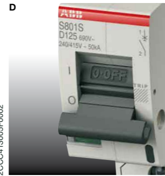
Tripping characteristics D Thermal tripping 1.13...1.45 \cdot I_n Electromagnetic tripping 10...20 \cdot I_n AC Calibration temperature 30^\circ\text{C}
