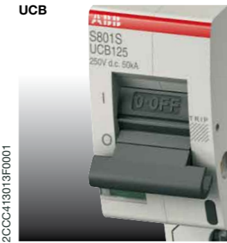
Tripping characteristics UCB Thermal tripping 1.05...1.3 \cdot I_n Electromagnetic tripping 6 \cdot I_n DC Calibration temperature 30^\circ\text{C}
