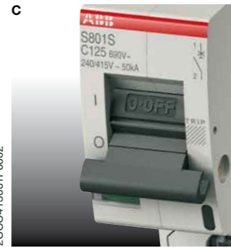
Tripping characteristics C Thermal tripping 1.13...1.45 \cdot I_n Electromagnetic tripping 5...10 \cdot I_n AC Calibration temperature 30^\circ\text{C}
